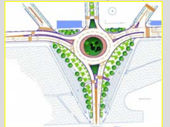
Passed layout (elliptic shape without "shunt lanes" for sake of a better landscape insertion)
