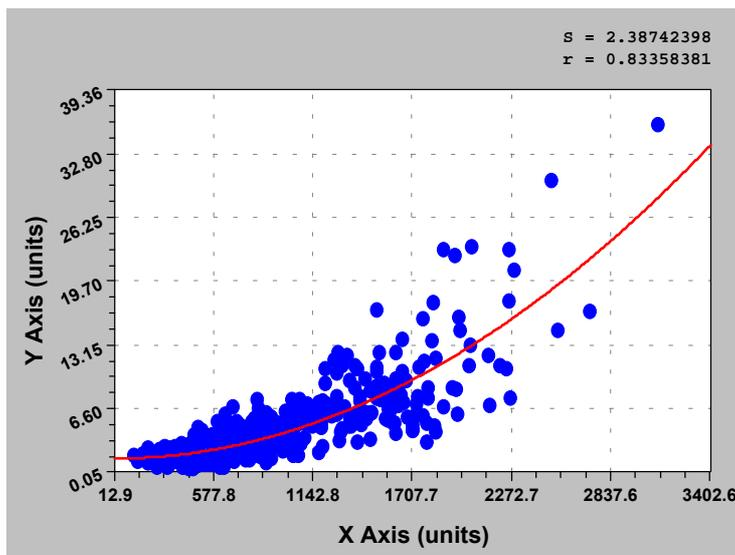
Fig. 5.2 Example for a best fitting altitude function (Climatic region: Alpine Region;  $a = 1.46 \text{ kN/m}^2$ ;  $b = 0.83 \text{ m}$ )
