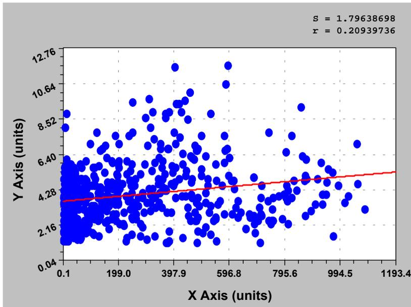
Fig. 5.4 Example for the absence of a clear altitude-snow load relationship (Climatic region: Norway;  $a = 3.60$ ,  $b = 2456$  m,  $r = 0.21$ )
