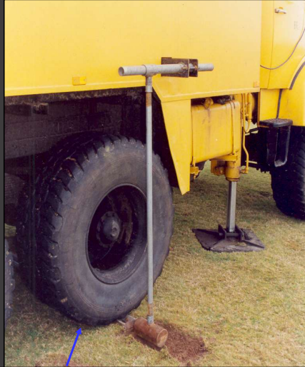
Normal force applied to beam for good contact with ground surface
