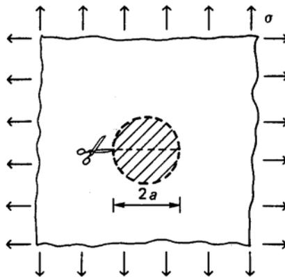
The elastic strain energy released is proportional to the strain energy contained in a circle of radius  $a$  (after Inglis):
