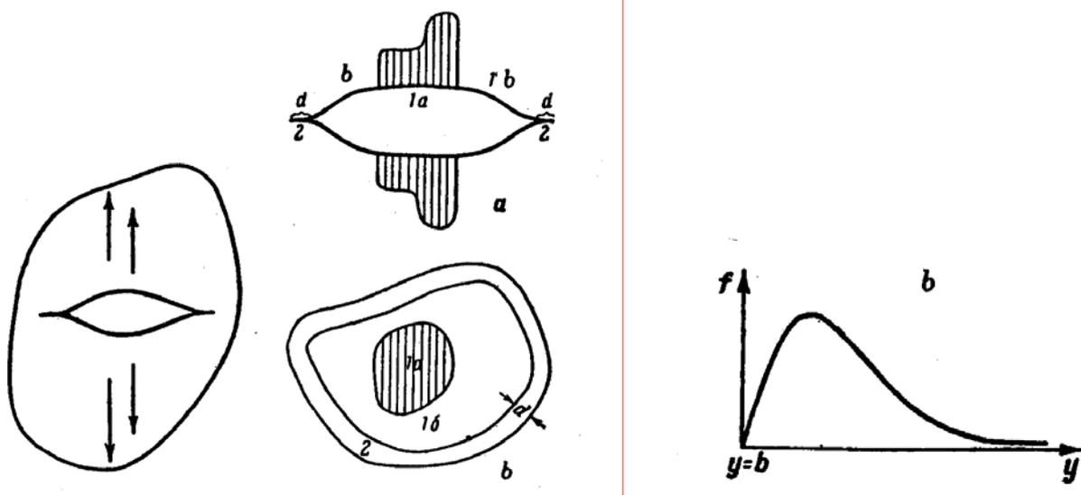
Represent the atomic bonds holding together the two halves of the body separated by the crack as cohesive forces acting along the edge regions of the crack and attracting one side of the crack to the other
