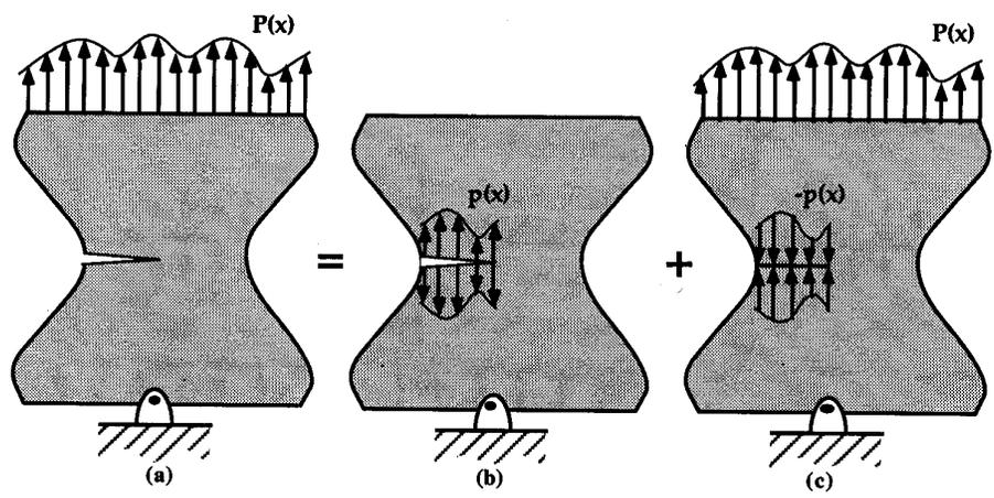
**Any loading configuration can be represented by appropriate tractions applied directly to the crack faces**
