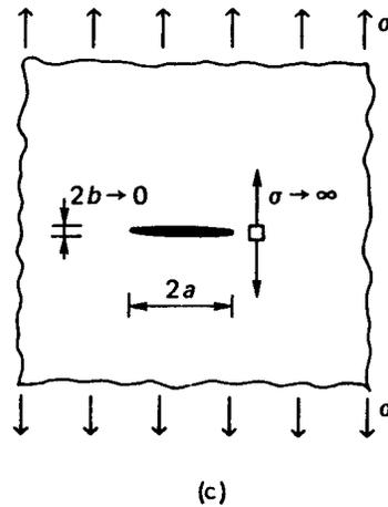
Plate with a crack: stress intensification at the crack tip
