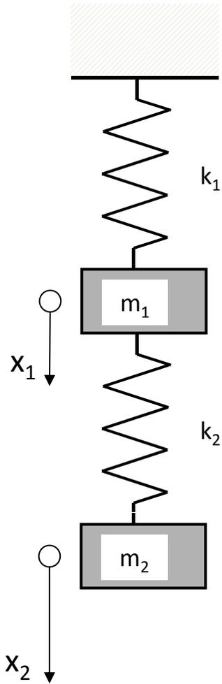
$$\omega^2 = \frac{\frac{3k}{m} \pm \sqrt{\left(\frac{3k}{m}\right)^2 - 4\left(\frac{k}{m}\right)^2}}{2} = \frac{k}{m} \frac{(3 \pm \sqrt{5})}{2}$$
