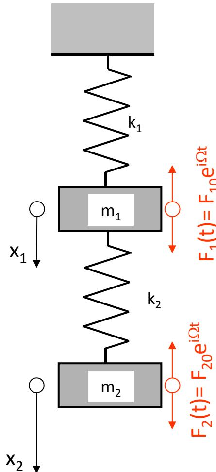
$$\begin{bmatrix} k_1 + k_2 - \Omega^2 m_1 & -k_2 \\ -k_2 & k_2 - \Omega^2 m_2 \end{bmatrix} \begin{Bmatrix} X_1 \\ X_2 \end{Bmatrix} = \begin{Bmatrix} F_1 \\ F_2 \end{Bmatrix}$$
